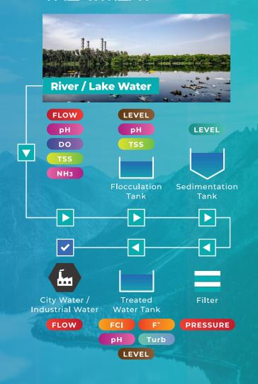
**Hydro-Air** provides total solution for applications from river water to ultrapure and wastewater monitoring.
